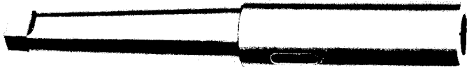
Figure 4-36 Steel socket used to hold twist drills with shanks too large to fit into either the drill press spindle or a sleeve.
